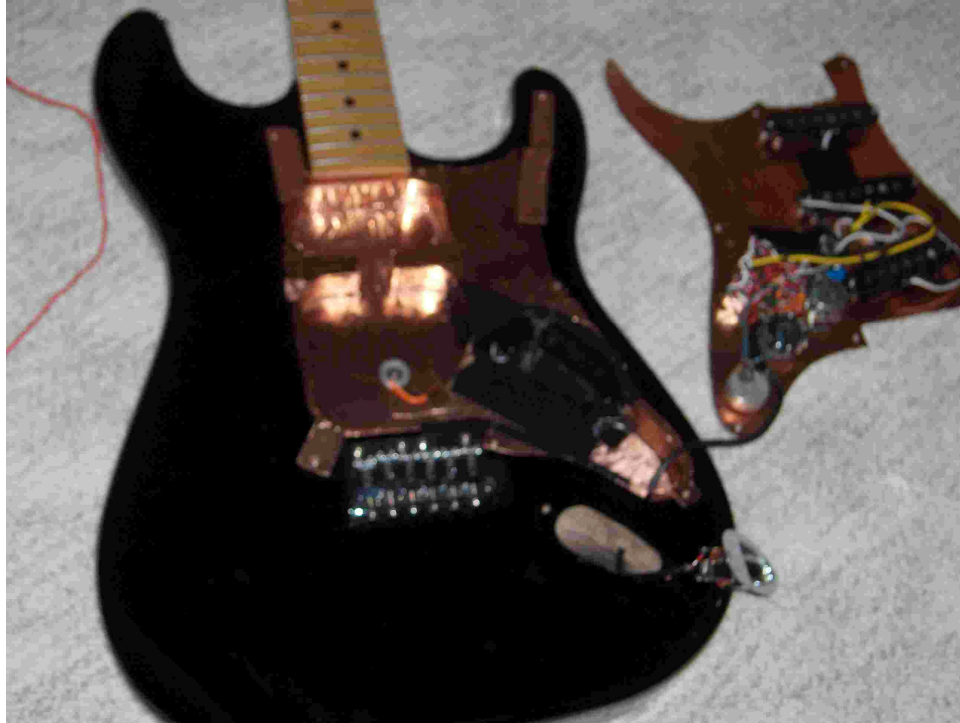
Figure 7. completed wiring, showing shielded stereo cable to input jack. Note black electrical tape to prevent accidental shorting against copper foil tape.
