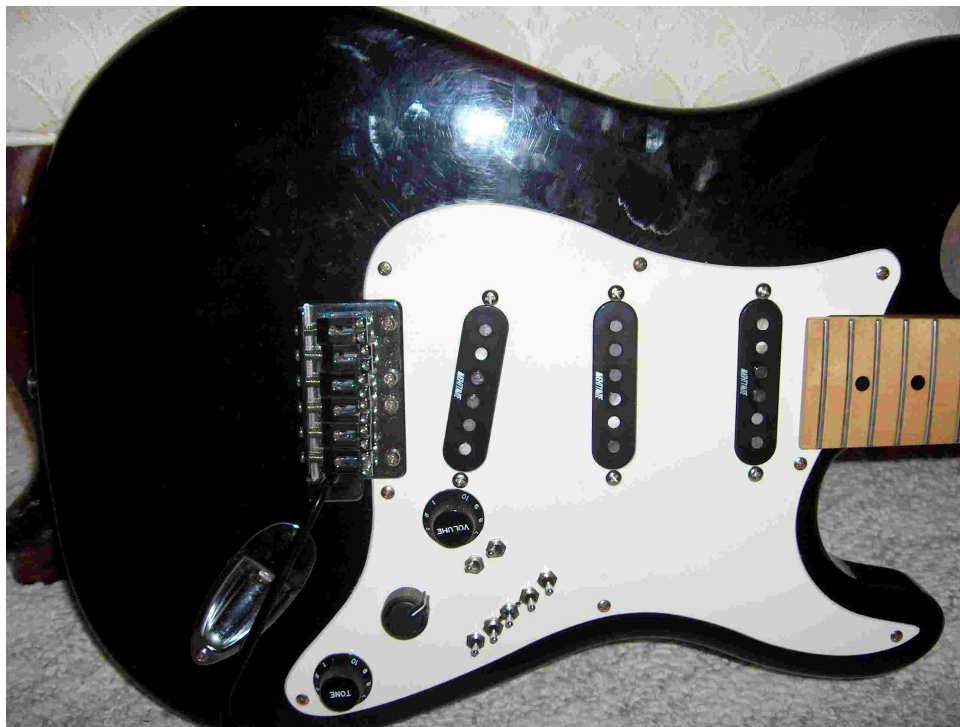
Figure 8. Job complete. Five SPDTs for pickup selection, bridge and neck DPDT phase switches, master volume, master tone, and 3-position tone select (0.047 \mu F, 0.022 \mu F, and open/no-load). You can get nearly any sound you want.
